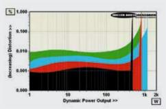
ABOVE: Dynamic power output versus distortion into 80hm (black trace), 40hm (red), 20hm (blue) and 10hm (green) loads. Maximum current is 28.3A
